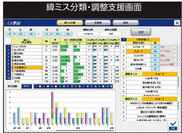
図7 緯ミス分類・調整支援画面 Fig.7 Weft Mispick Stratification & Adjustment Support Screen
