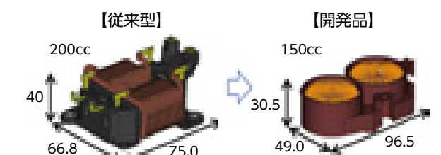
図7 PFCコイル従来型と開発品の比較 Fig.7 Comparison the current type PFC coil with the developed type PFC coil
