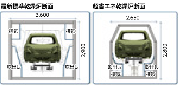
図18 乾燥炉断面比較 Fig.18 Comparison of cross sectional view, Regular oven / energy conservation oven
