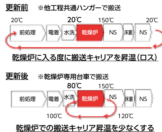
図12 搬送キャリアの動きと温度推移 Fig.12 Behavior of carrier transportation and temp. transitive
