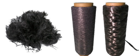
図4 使用済みCFRPの再生炭素繊維とその紡績糸 Fig.4 Recycled Carbon Fiber and its Spun Yarn
