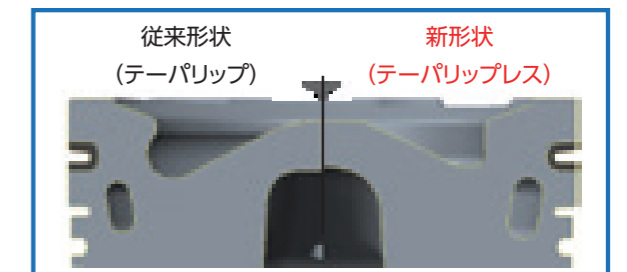
図7 燃焼室形状 Fig.7 Combustion chamber shape
