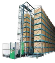
Automated Storage and Retrieval System for Pallet Rack Sorter P
