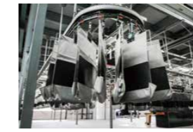
Hanging Type High-Speed Sorting System Pocket Sorter
