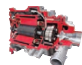
Air Compressor used in the Mirai
