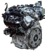
A25A-FKS Displacement: 2.5 liters used in the RAV4
