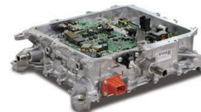
Integrated On-Board Charger and DC-DC Converter Unit
