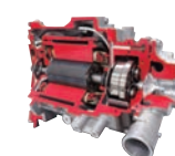
Air Compressor used in the Mirai
