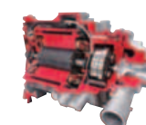
Air Compressor used in the Mirai
