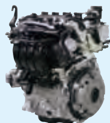
M20A-FKS Gasoline Engine (Displacement: 2.0 liters, used in the RAV4 and Corolla Sport)
