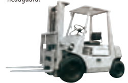
Lift truck with built-in headguard
