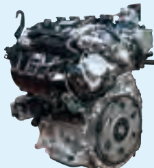
A25A-FKS Gasoline Engine (Displacement: 2.5 liters, used in the RAV4)
