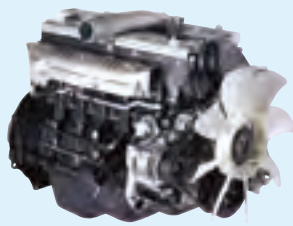
1HZ Diesel Engine (Displacement: 4.2 liters, used in the Land Cruiser)
