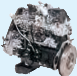
2KD-FTV Diesel Engine (Displacement: 2.5 liters, used in the Hiace)
